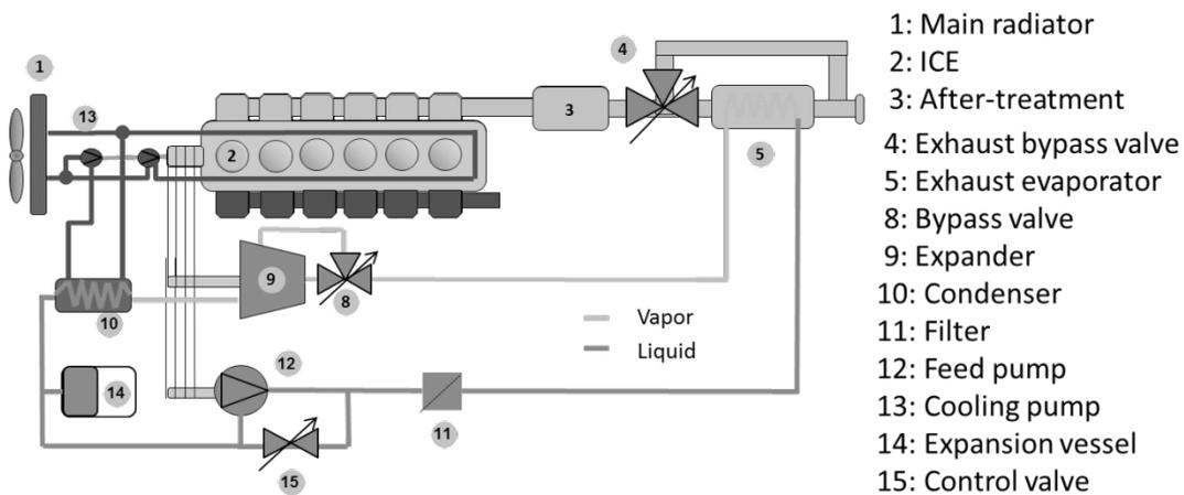
Fig. 1. ORC system considered for this business case (turbocharger is not shown)
