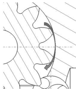
**Figure 4:** Leak path at gears teeth periphery
