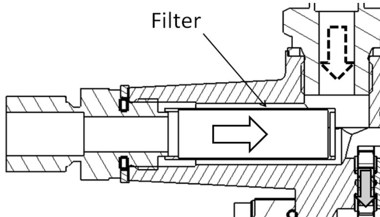
**Figure 14:** plain arrow is the flow coming from the condenser, and dash arrow is the fluid controlled in pressure thanks to the expansion vessel located just above.
