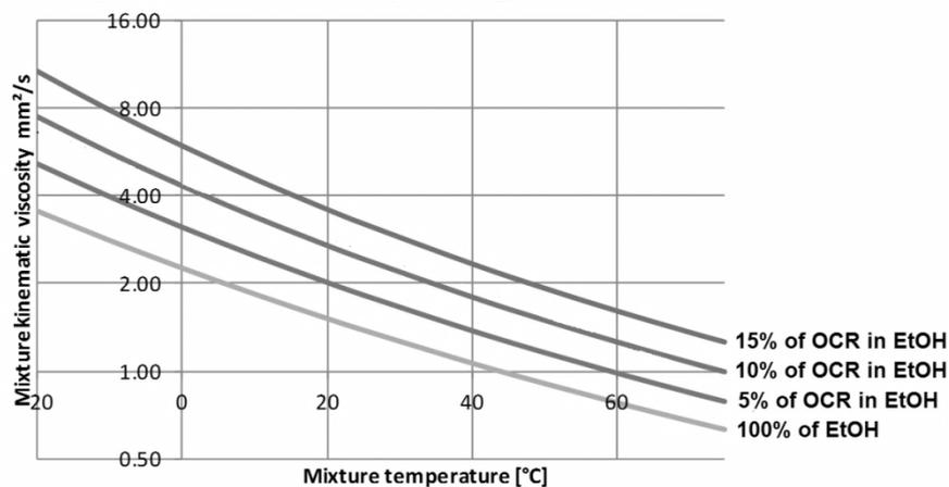
Figure 11: kinematic viscosity of ethanol with several different oil percentages
