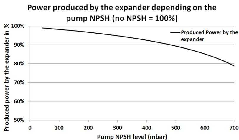
**Figure 15:** expander relative performance (in %) depending on the pump NPSH level.
