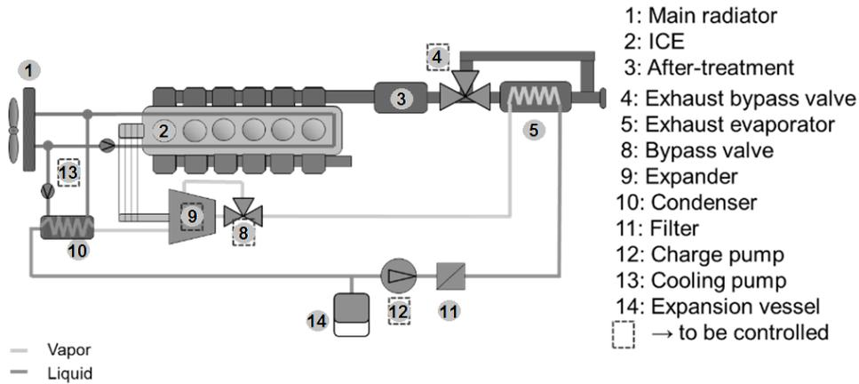
Figure 1: Organic Rankine Cycle system for a heavy truck
