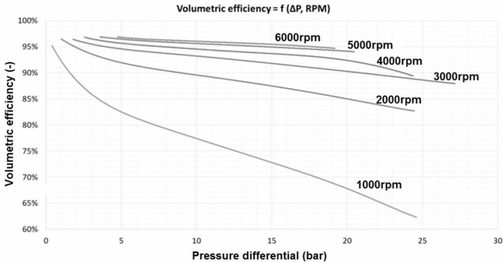
Figure 10: influence of the pump speed and pressure differential on the volumetric efficiency
