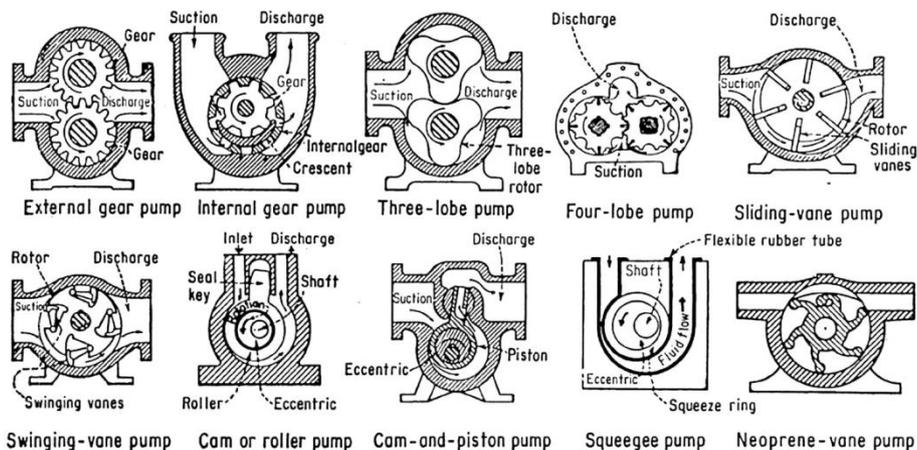
Figure 3: types of displacements pumps. Suction area is the LPA, whereas discharge is HPA.
