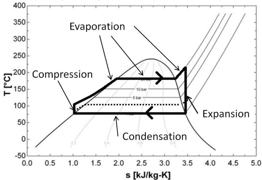
**Figure 13:** T-S diagram for a typical Rankine cycle (plain).
