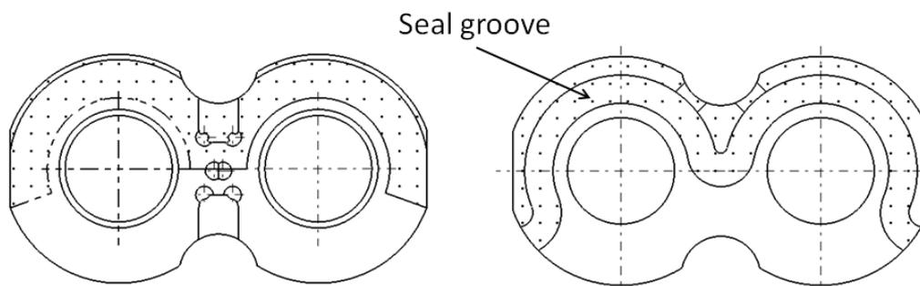
**Figure 6:** floating compensation plate design.
