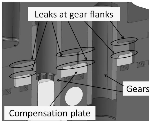
**Figure 5:** Leak path at gears flanks
