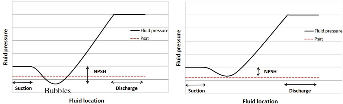
**Figure 12:** Left graph: fluid pressure goes below  $P_{sat}$  (=saturation pressure), cavitation occurs. Right: NPSH is lower, fluid pressure remains above  $P_{sat}$ . No cavitation occurs.
