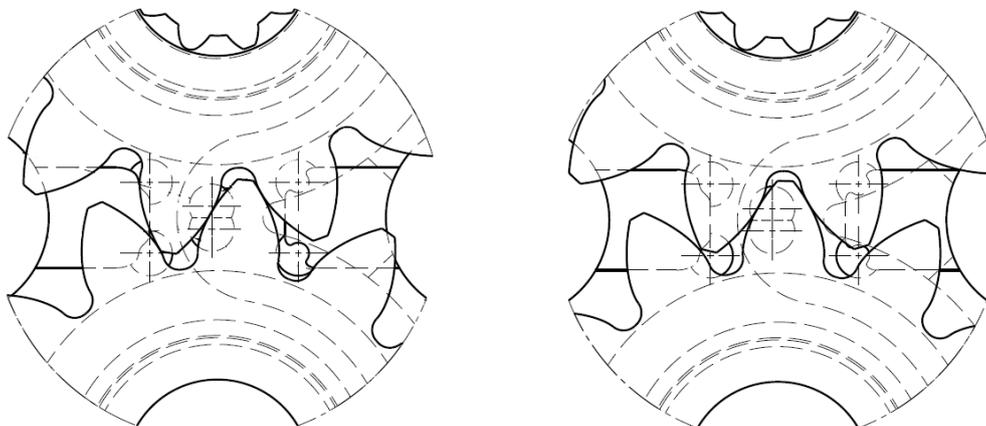
**Figure 9:** gears interface cavities for 2 gearing positions
