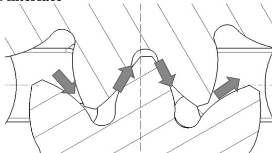
**Figure 8:** Leak path at gears interface
