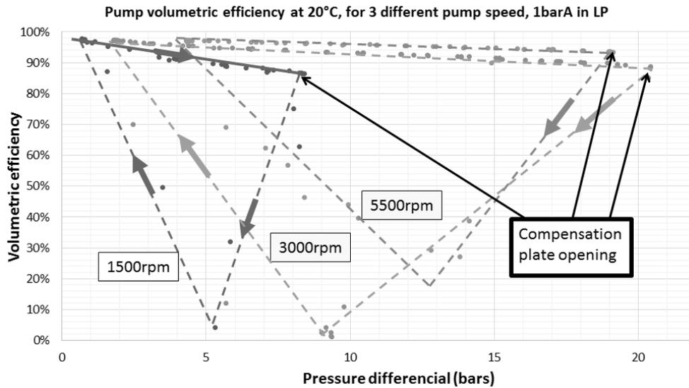
**Figure 7:** example of a compensation plate which opens the circuit (HPA too small on casing side)
