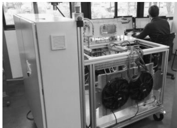
Figure 2: Photo of a version of the test stand equipped with a radiator with fans
