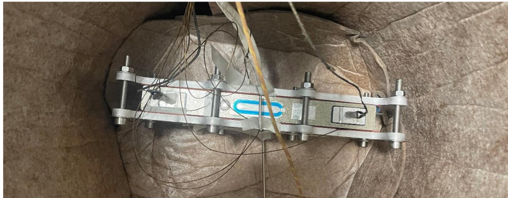
NMC 92 cell before cell abuse test
